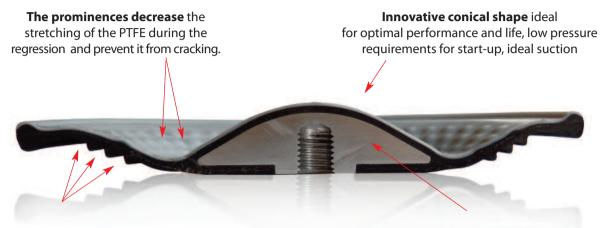
Innovative diaphragm support side, offers flexibility, long life and protects from cavitation **Special internal plate** supports your diaphragm in every movement
